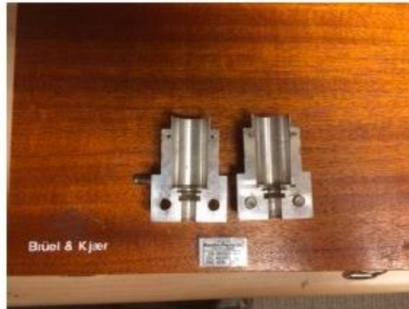
Exhibit 2: Pistonphone and Coupler Used to Calibrate Hydrophone (top: calibrator and coupler, bottom: coupler disassembled)
