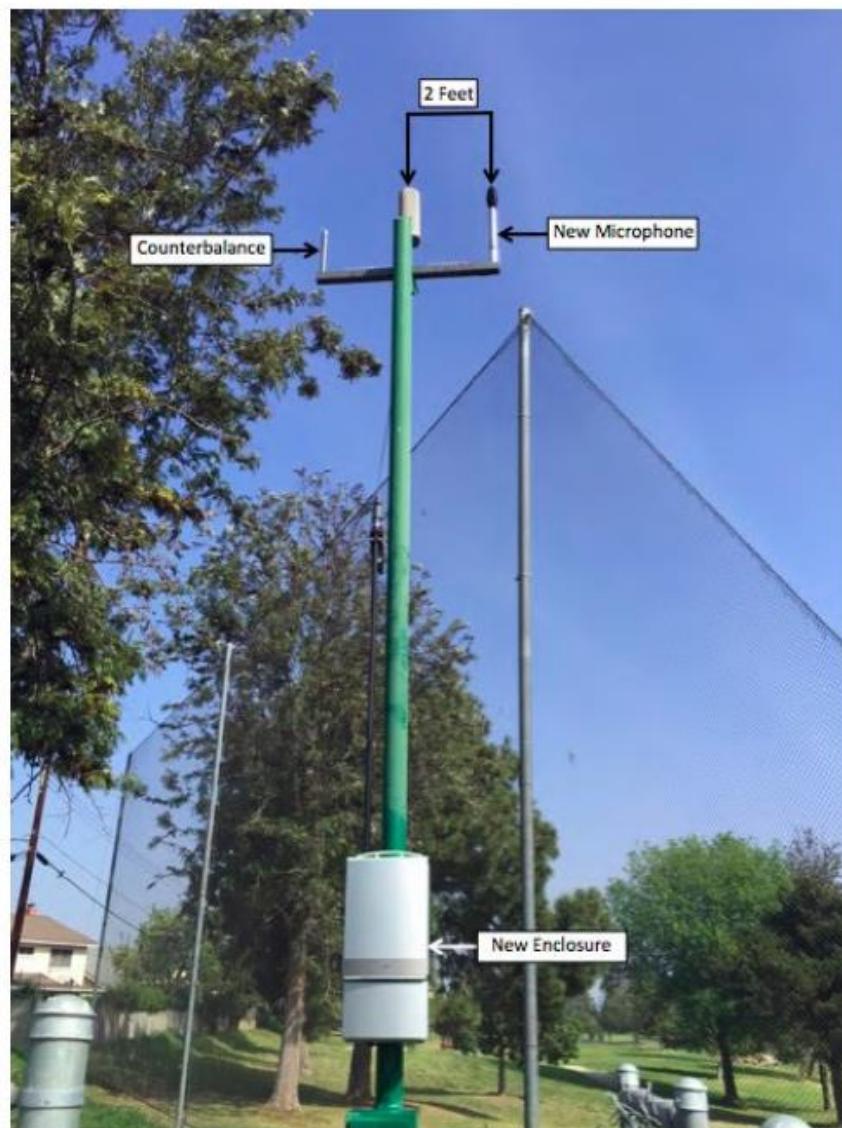
Exhibit 3: Sketch of Microphone Setup
