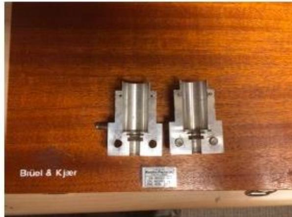
**Exhibit 2: Pistonphone and Coupler Used to Calibrate Hydrophone
