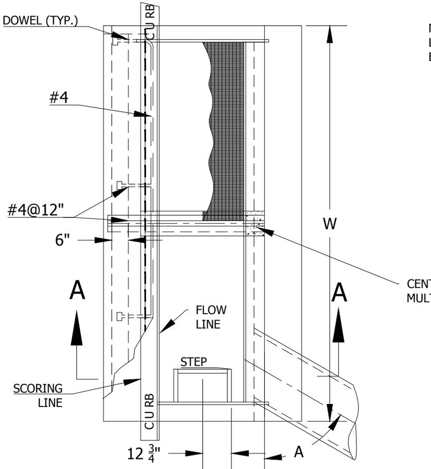
NOTE: GRATE SHALL BE LONG BEACH IRON WORKS LB24-10C WITH GALVANIZED FINISH OR APPROVED EQUIVALENT.
