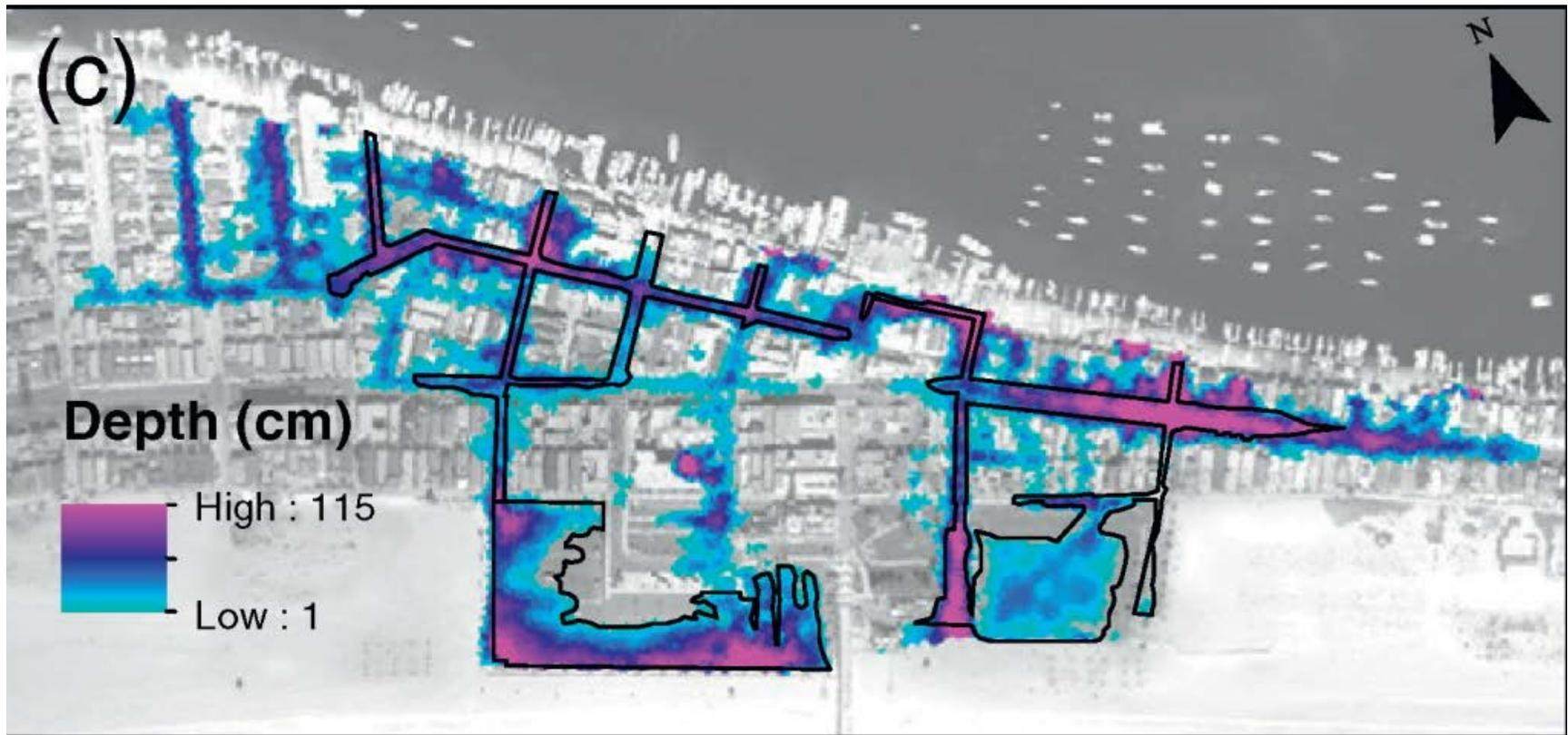
**Figure 4.** Observed flood extent (solid black line) vs. flood extent predicted using the HR and BreZo modeling methodology, for the August 2011 wave overtopping event at Newport Beach. Extracted from Gallien et al. (2014).
