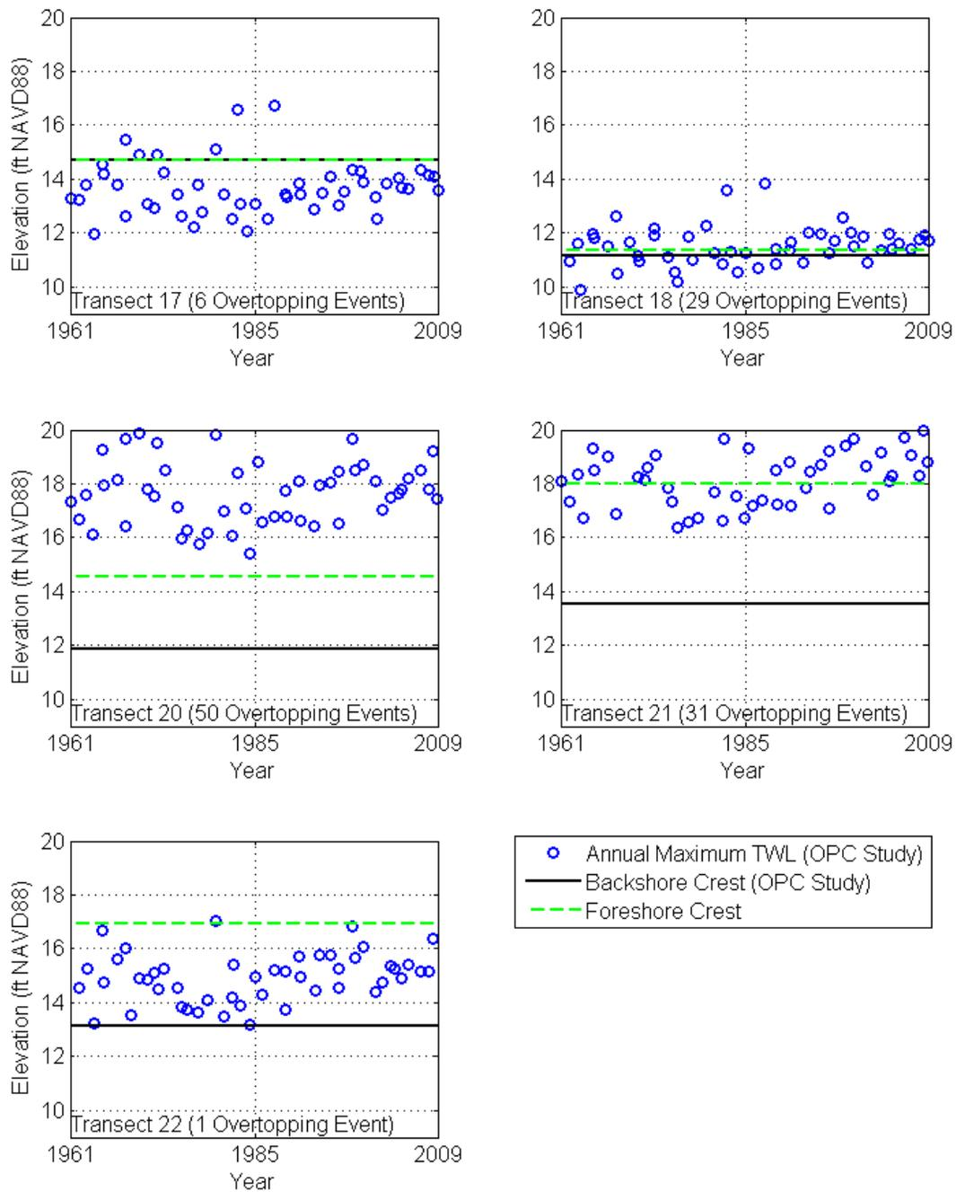
**Figure 1.** Comparison of OPC Study TWLs to foreshore beach crest elevations and selected backshore feature elevations for Transects 17, 18, 20, 21, and 22. Projection of the annual maximum TWL to the backshore crest would result in flooding of properties at least every year from 1961 – 2009 for Transects 18, 20, and 21.
