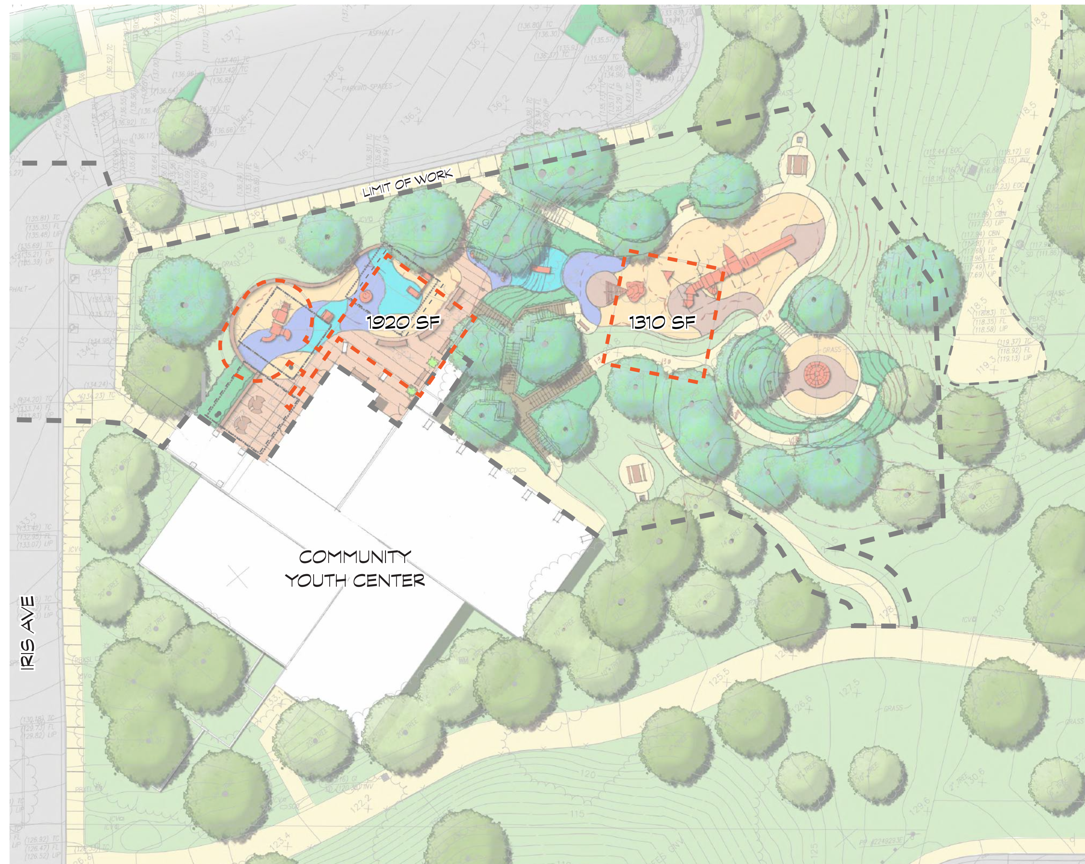
CONCEPTUAL PLAN: EXISTING PLAYGROUND AREAS (3,230 SF) VS. IMPROVED PLAYGROUND AREAS (4,695 SF) SCALE: 1" = 20'-0"
