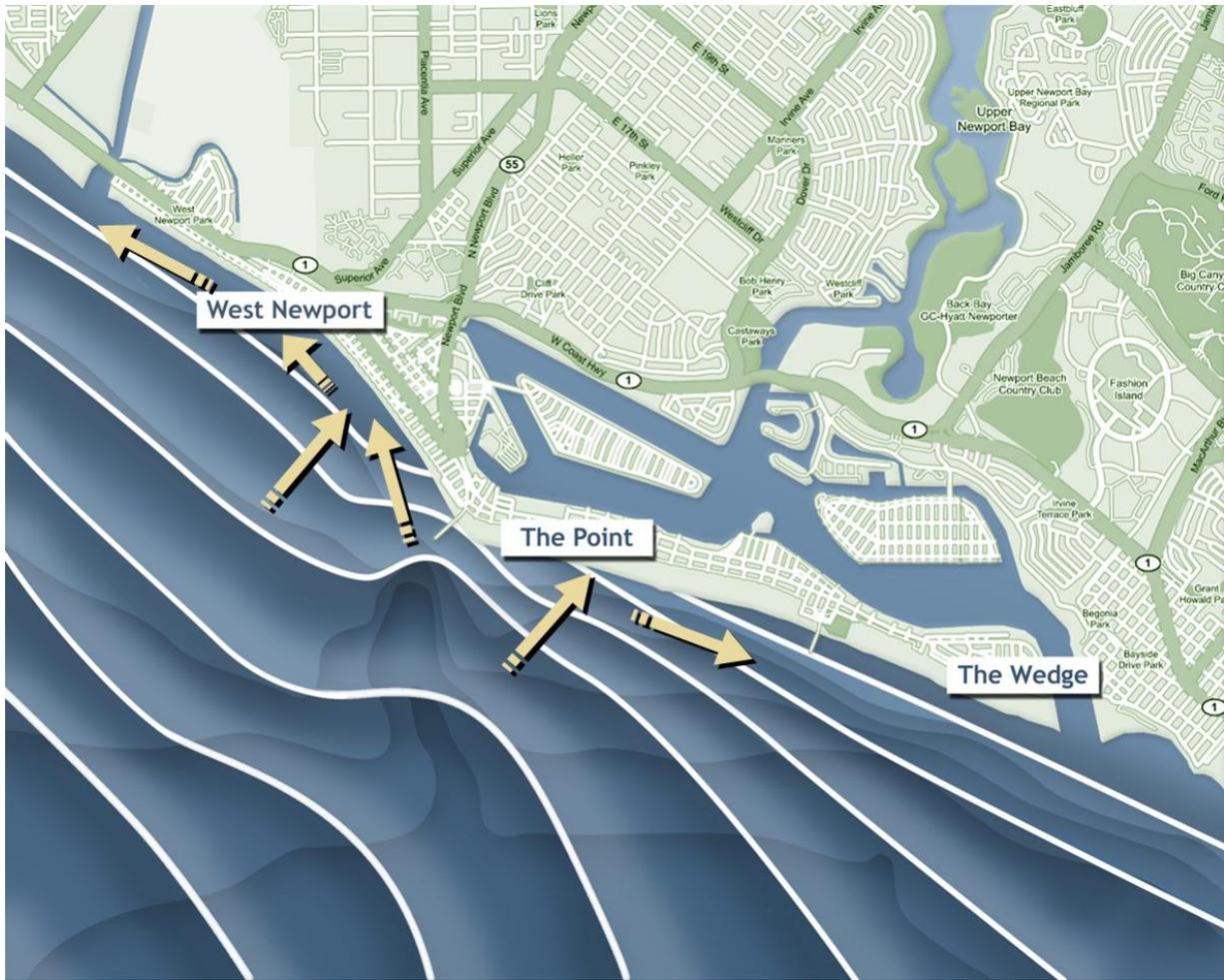
Figure 2-3: Wave Refraction during Southern Swell
