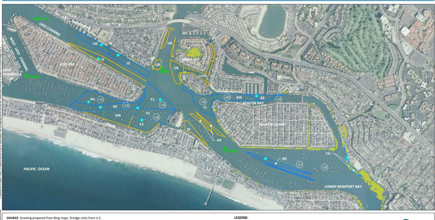
SOURCE: Drawing prepared from Bing maps. Dredge units from U.S. Army Corps of Engineers. HORIZONTAL DATUM: California State Plane, Zone 6, NAD83. VERTICAL DATUM: Mean Lower Low Water (MLLW).
