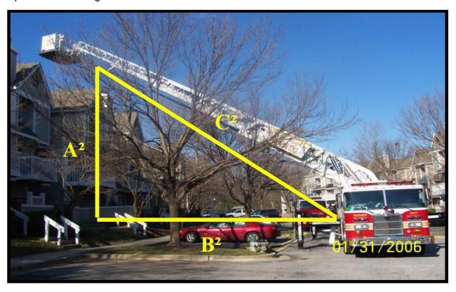
In this illustration, "A" equals the height of the building (use 12 feet per floor for commercial and multi-family structures). "B" equals the distance from the building to the turntable. "C" is the required distance to reach the building.
