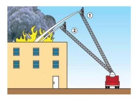
Aerial positioning is dependent on many factors such as access, type of structure, primary objectives, hazards, obstructions, and most importantly the reach of the aerial ladder. This determination of positioning will be subject to a case-by-case basis but at a minimum the quint or ladder truck has a minimum of  $^{\odot}$ 15-feet and a maximum of  $^{\odot}$ 35-feet from the building. This gives the ladder the greatest load capability when maintained between 40 to 75 degrees.
