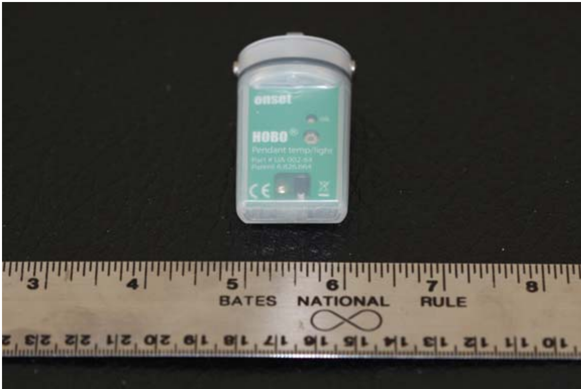
Photograph 5 . A HOBO Temperature and Light Pendant Data Logger That Measures Light Intensity (lumens per foot 2 )
