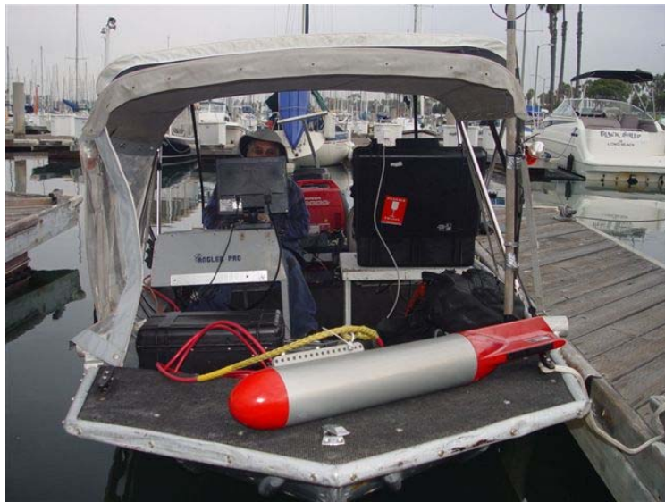
Photograph 11. Imagenex 881 Sportskan Sidescan Sonar Towfish
