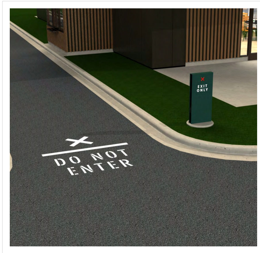
Ground Graphics are to be either Thermal applied or stenciled and painted white.
