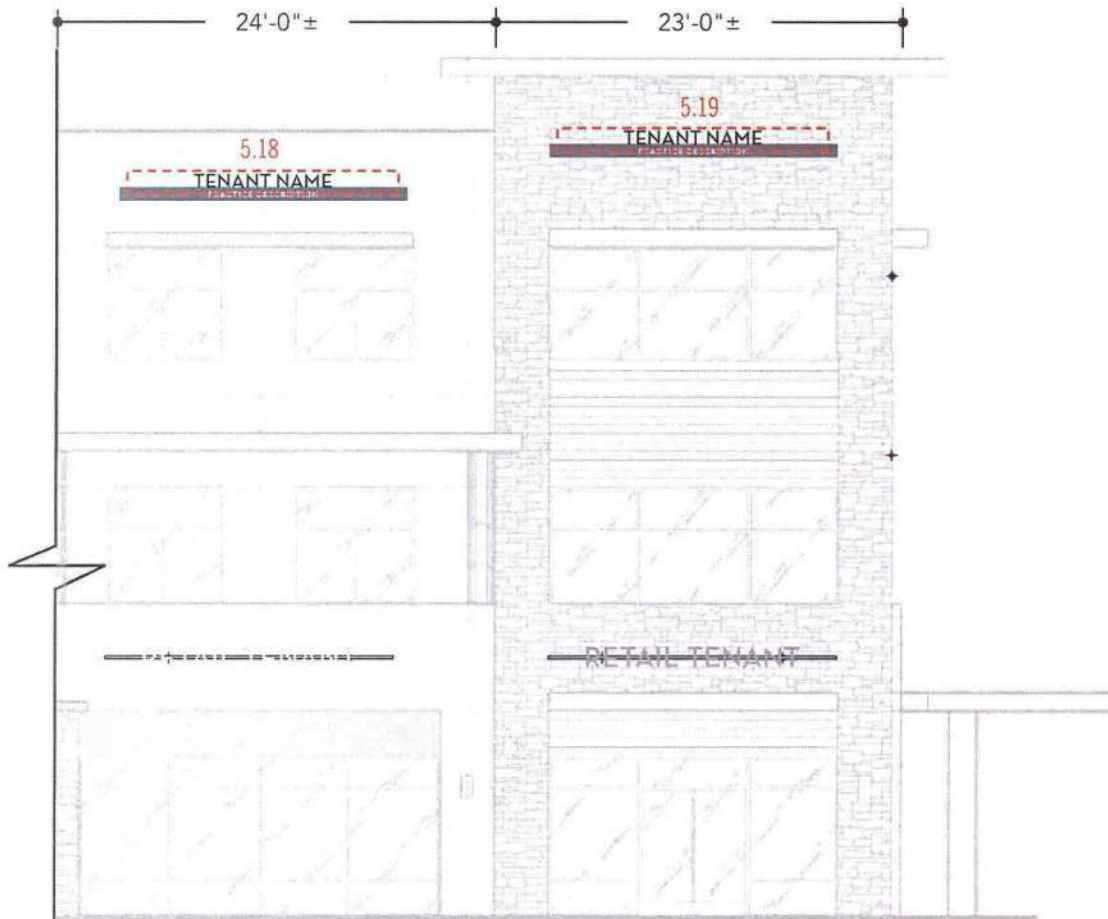
BUILDING 4: NORTH ELEVATION B SCALE: 3/32" = 1'
