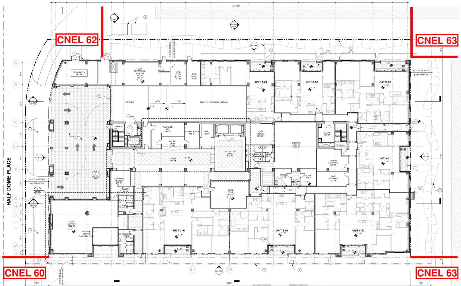
Figure 5: Predicted Community Noise Equivalent Level (CNEL) contours on first floor
