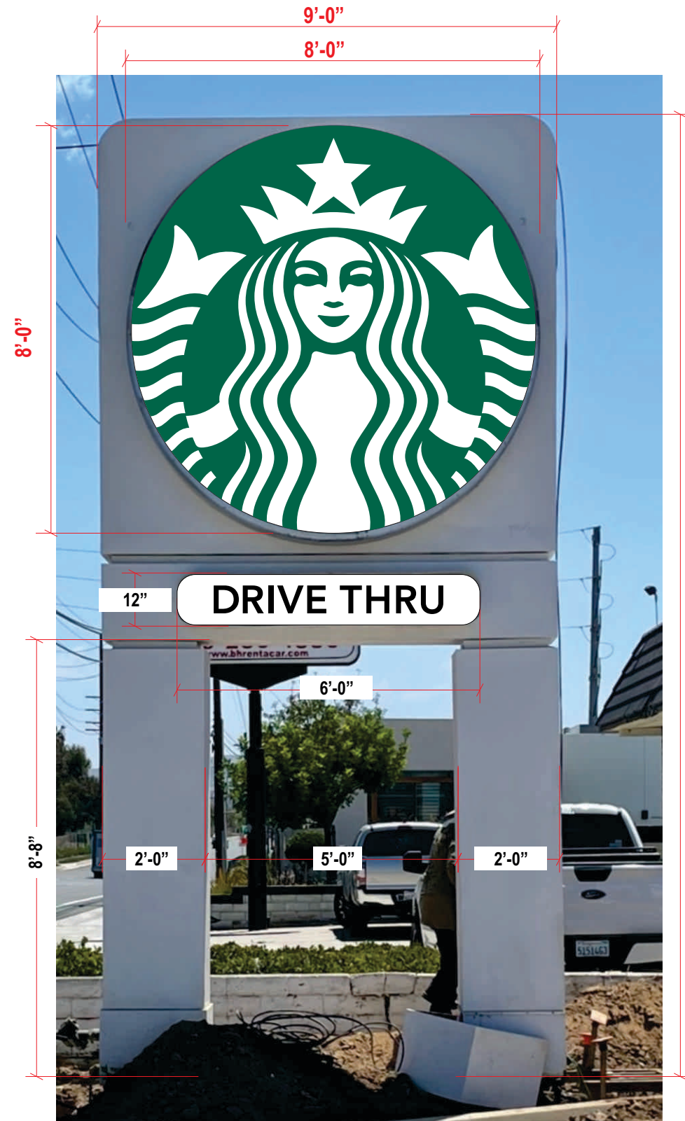
EXISTING PYLON SIGN - PROPOSED SIGNS
