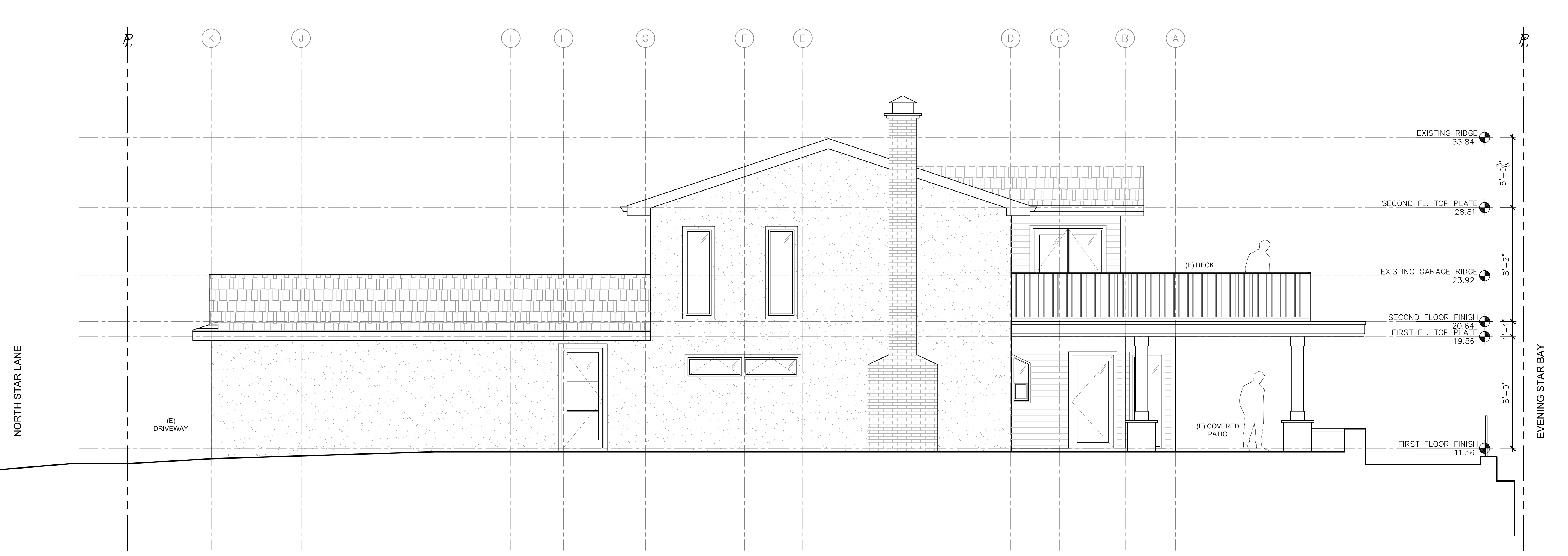
2 NORTH ELEVATION EXISTING 1/4" = 1'-0"
