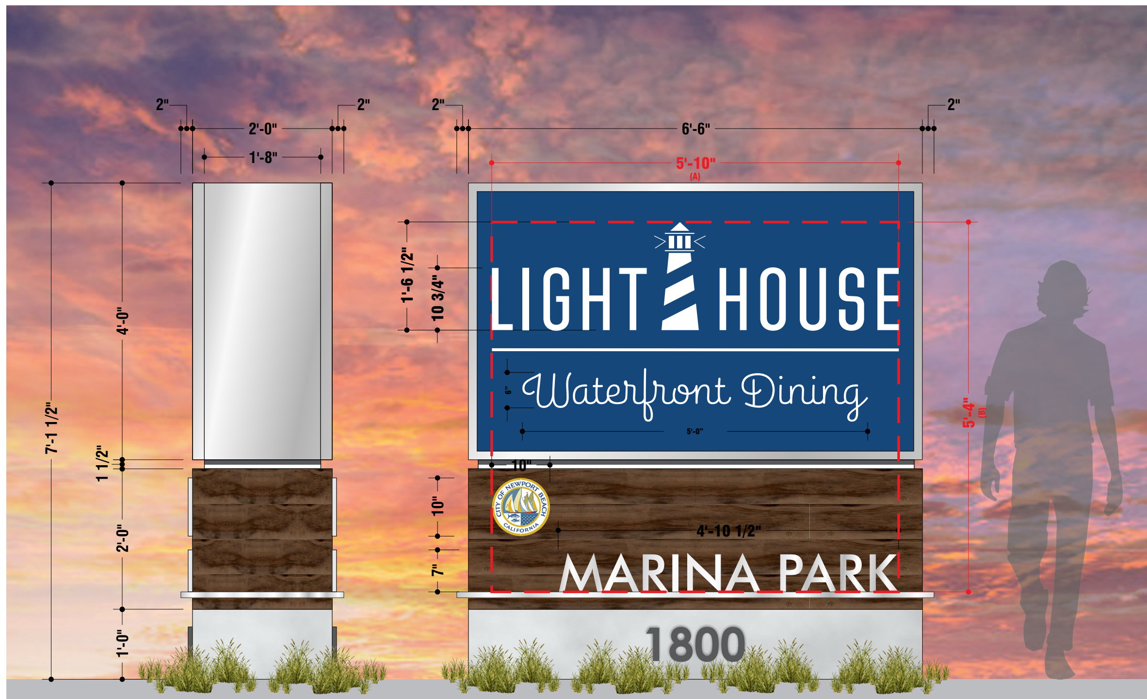
7A SIGN F / NEW PROPOSED NON-ILLUMINATED D/F MONUMENT SIGN SIZE DIMENSIONS scale: 3/4"=1'-0"
